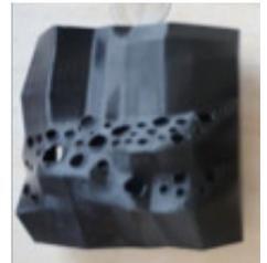
*The prototypes were made using a Makerbot 3D printer at the Fab Lab XCHC in Christchurch. The final designs are white and bone color, black would hold in too much heat from the sun, which is not ideal for the plants nor for the durability of the planter panels.*
